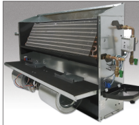
End Pockets The 7.5" end pockets allow for accessibility and service of optional factory piping packages and controls. End panels are removable to allow for even greater access.
